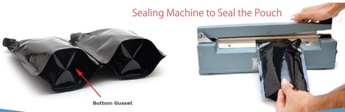
Place the Funnel on the top open area of the pouch to fill in Liquid Product, then seal the pouch
